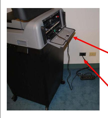
Unlock wheels and turn the DS200 around. Using silver key, unlock the back door compartment.
