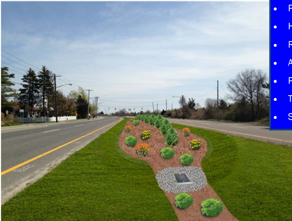
A conceptual photo-simulation showing the redesigned median and an aesthetically-pleasing landscaped berm to accommodate stormwater runoff.
