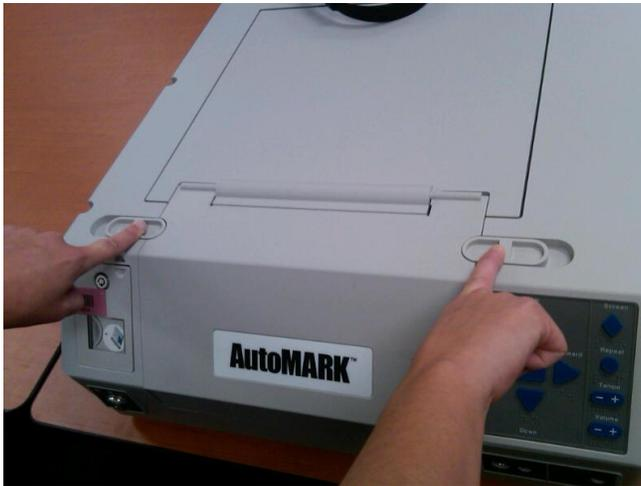
Slide the plastic clips towards the center to secure
