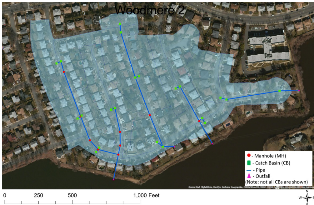
Figure 13: Woodmere2 (N4) Drainage Area
