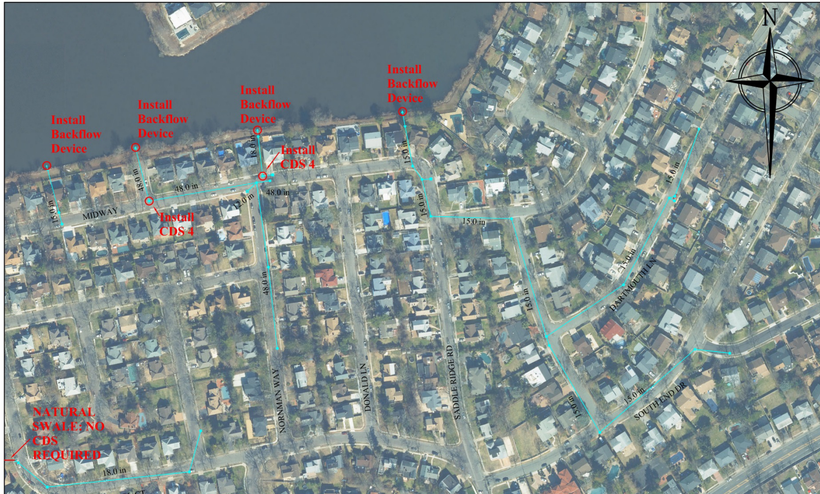
Figure 17: Woodmere3 (N5) Plan 1 – Backflow Prevention (4 of 16 outfalls)
