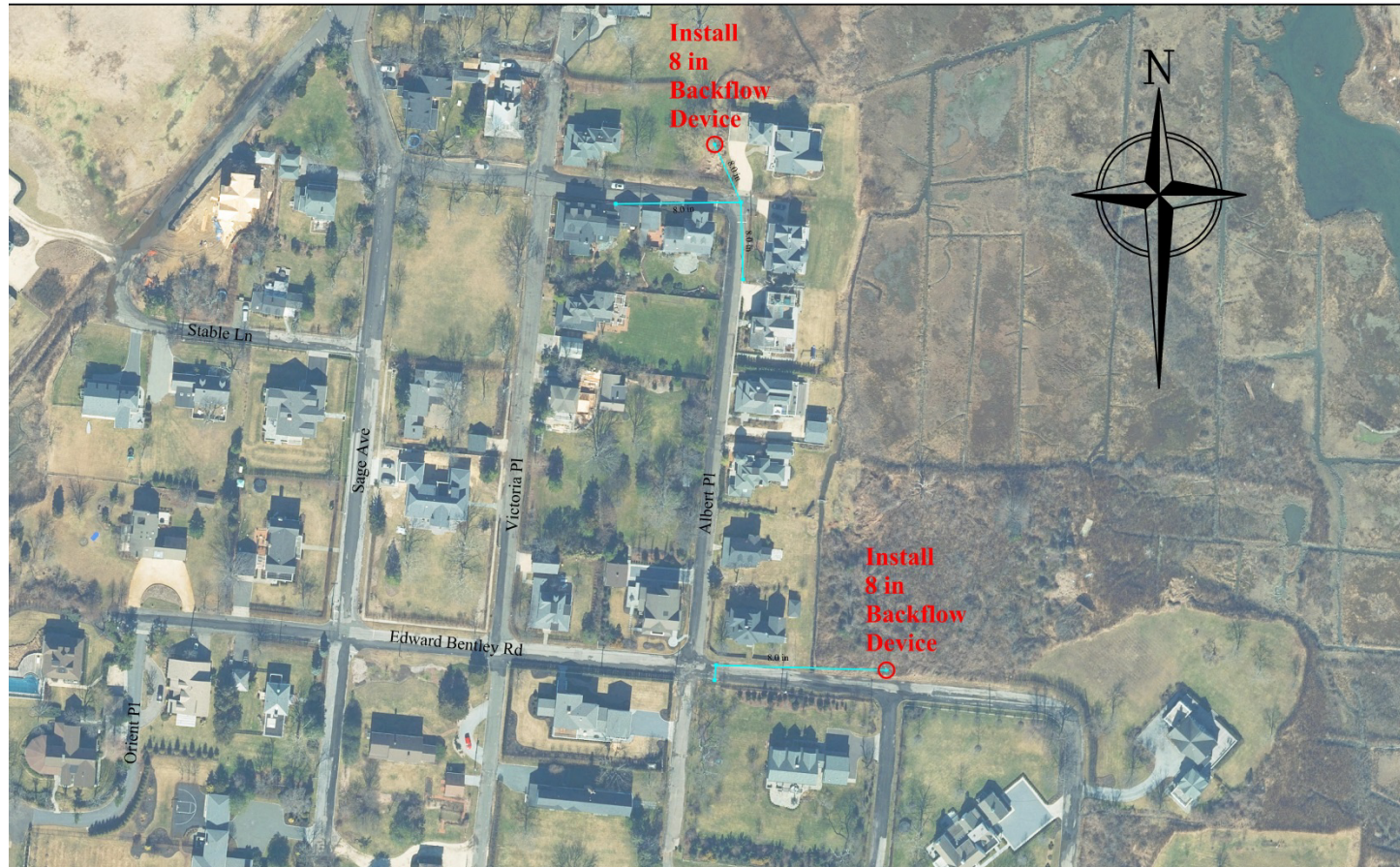
Figure 25: Lawrence Plan 1 – Backflow Prevention at Albert Place
