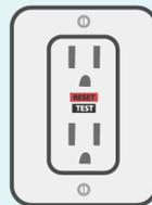
Install **GFCIs**, which can prevent electrocution, on all receptacles within **20 feet** of water's edge.
