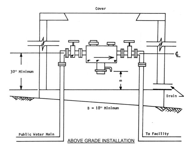
The improper installation of these devices can negate the desired protection. Most critical is the need to provide a gravity drain large enough to receive the maximum potential discharge of the relief valve. This drain cannot be subject to flooding and must be screened.
