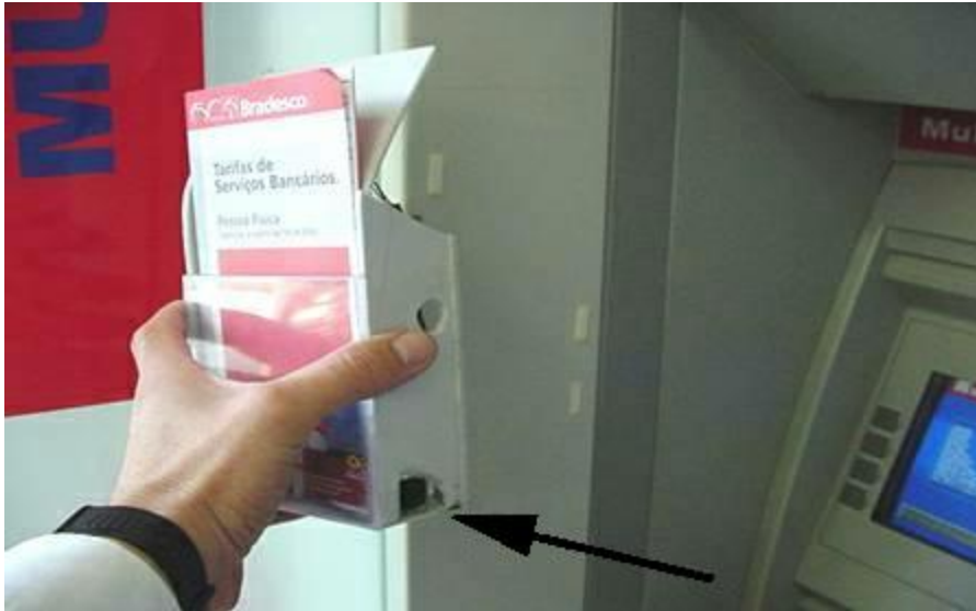
The PIN reading camera being installed on the ATM is housed in an innocent looking leaflet enclosure.
