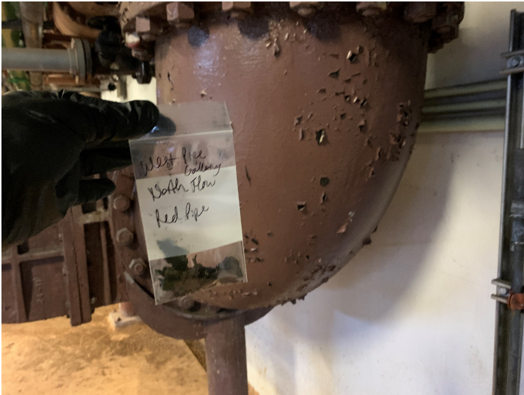
West Pipe Gallery: LCM* North Flow Red Pipe Paint
